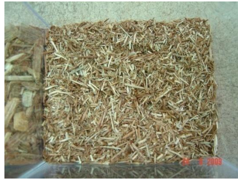
Wood particles after Hammer mill.
